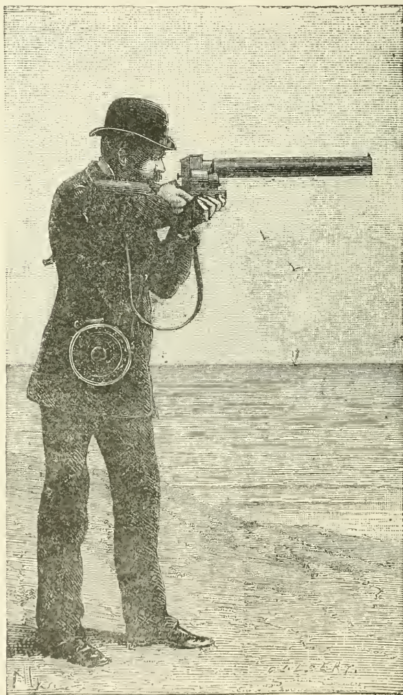
FIG. 17. MODE OF USING THE PHOTOGRAPHIC GUN.
